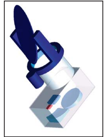
3D concept of the OSDT instrument with an additional scanning mirror to allow the detection / tracking of very fast debris particles (up to 15km/s).
